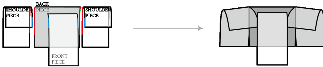
Fig.18 The front view structural drawing of Blue Trousers Yao Guanshou costume (Red imaginary line: fold line; red and blue full line: sewing line)
