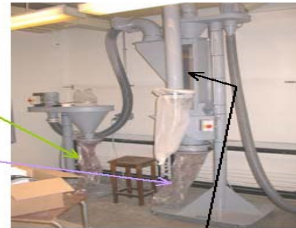
(3) Waste separated into fibrous and granular components
