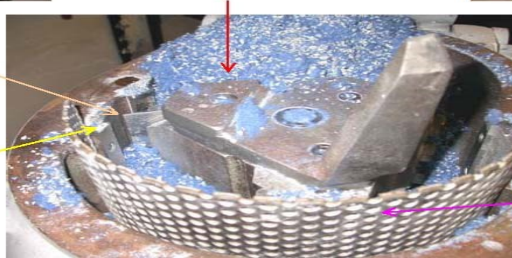
(2) Tiles shredded in granulating chamber and conveyed by suction through screen
